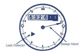
Wait an hour or more without using any water in your home and read your water meter again. If the sweep hand has moved, something has used water. To determine the amount of water unaccounted for, subtract the first reading you noted from the second reading. The result is the amount of water measured between readings.
